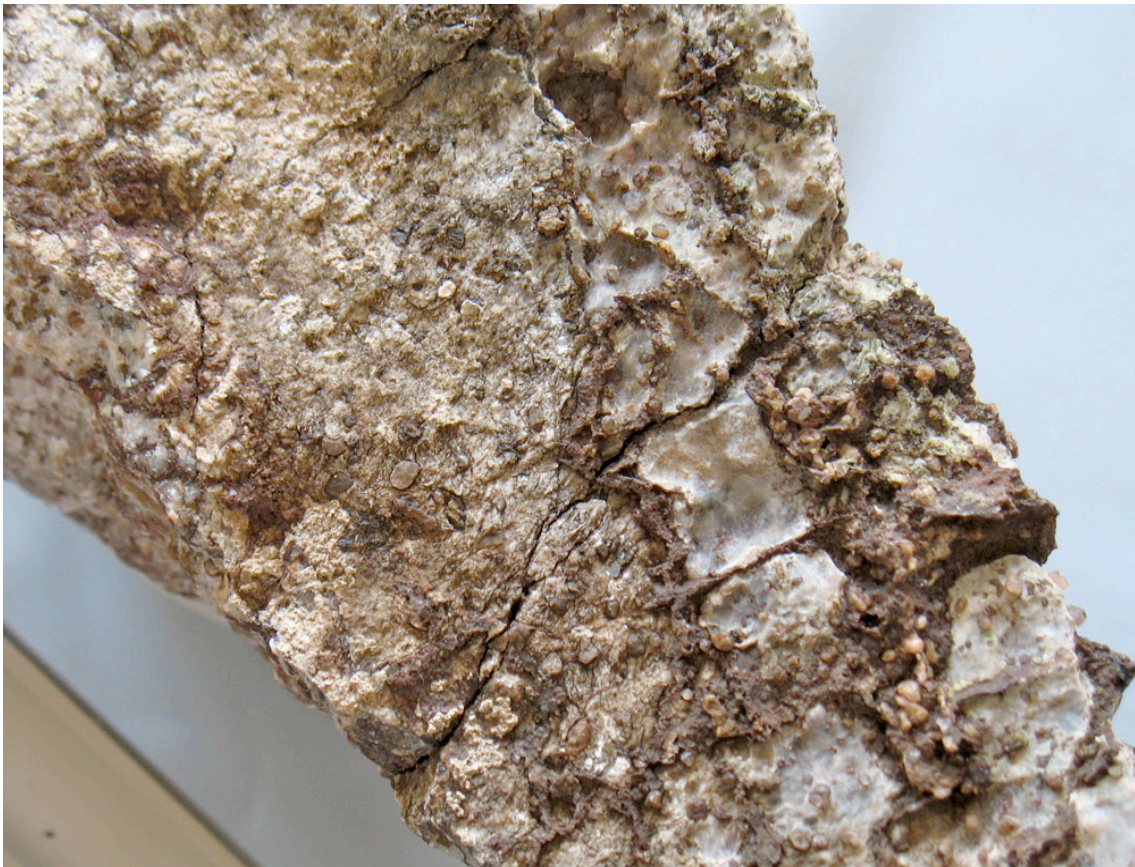
Fig. 22: Backside of Fig.20. A brown melt is clearly visible in the right part, (2589)
